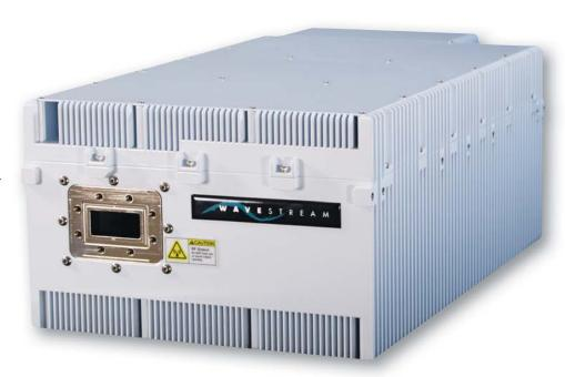
The 500W SSPA takes high efficiency to a new level in solid-state power amplifiers. Wavestream's proprietary spatial power combining enables packing 500 Watts into a rugged 85-lb. unit that can be mounted directly on medium aperture antennas, maximizing the power into the feed and further enhancing system-level efficiency.
